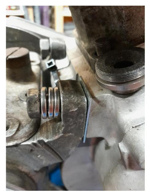
7. Then I dismantle the whole thing again until final assembly. During final assembly, make sure that the seals between the primary and the engine or gearbox housing are of the same thickness.
