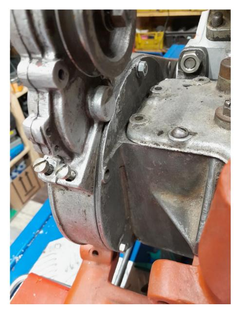
4. In most cases you will then find that not all 4 retaining arms of the gearbox are evenly in contact with the engine, although the primary firmly connects the engine and the gearbox.
