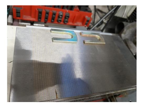
6. I then detach the primary from the engine and gearbox, insert the prepared washers between the gearbox and engine and tighten the gearbox.The gearbox should be easy to assemble and lie absolutely flat on the engine.After that, the primary should fit easily and without tension on the centering collars during assembly and completely rest on the plane surfaces of the engine & gearbox.
