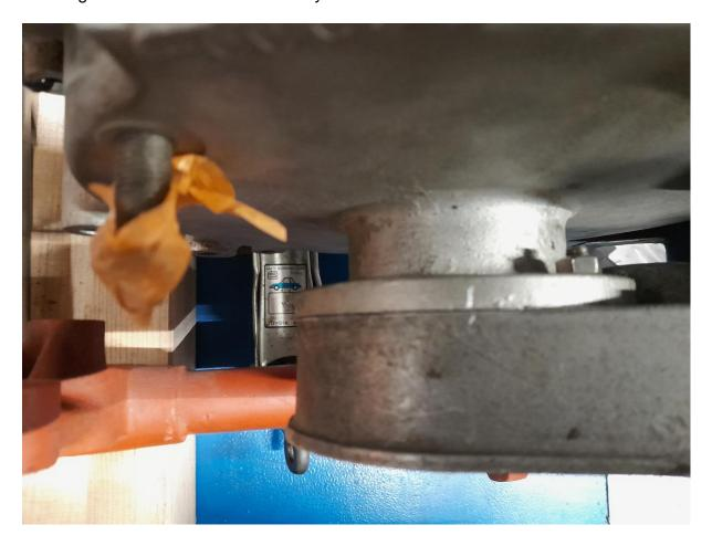
2. Loosely screw the engine and gearbox together so that the gearbox can still be moved.
